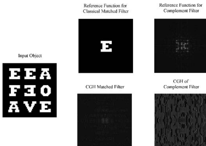
Figure 23.37 Input object, reference function, and CGH for the classical matched filter, and edge-enhanced reference function and CGH for the complementary matched filter. Note the additional high-frequency information transmitted by the latter CGH.
